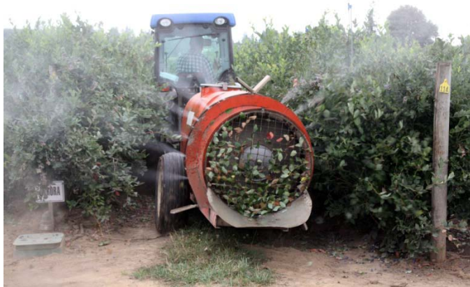
Fig. 1. Airblast sprayer application to mature 'Aurora' blueberry, 50 gpa at 100 psi.
